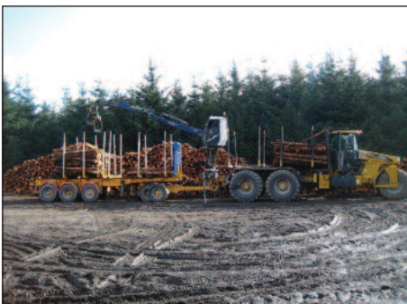
Low ground pressure (LGP) haulage
